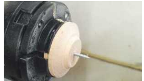
▲ Pic.6 To make the hat, mount up a small screw chuck; this is ideal as the hat will need a hole in it and you can utilise that to hold onto
